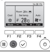
Press the **RETURN** button to exit the Main menu and return to the Main display.
